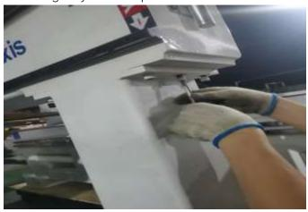
2. Connect Z axis motor and z axis dragchain
